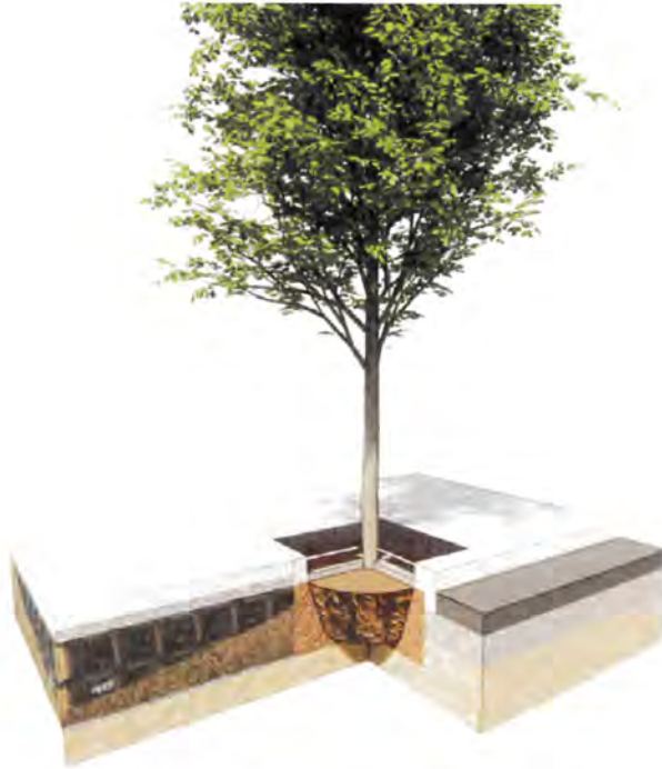
OPTION 2: Structural soil support cells and tree grate
