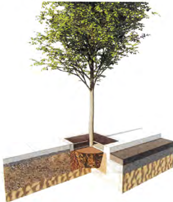
OPTION 2: Structural soil support cells and tree grate
